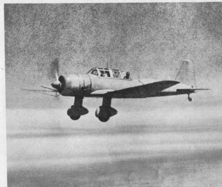
SONIA Though obsolescent, Sonia is still operational, particularly against Chinese ground forces. Landing gear, wing dihedral on outboard panels only are important recognition aids.
